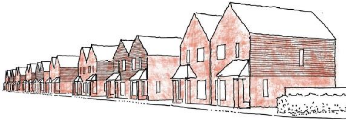
Sketch of use of projecting brickwork to provide articulation along street frontage
